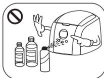
Do not fill the tank with abrasive or corrosive chemicals.
