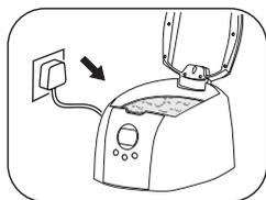
Please ensure that the device is switched off and remove the mains plug from the socket.
