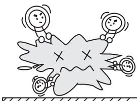
Many tiny bubbles are created when ultrasonic sound is passed through liquid.
