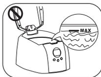
Keep the unit unplugged before filling. Do not fill water above "MAX" line of tank.
