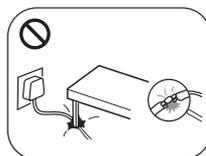
Never operate this unit if the plug or cord is damaged. Please refer to a service centre for examination and repair.
