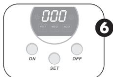
After the set time has elapsed the cleaning process is automatically stopped, the blue indicator lamp goes off and the display shows 000.
