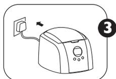
Close the cover and insert the mains plug. The figure 180 (180 seconds) appears in the display as standard - this is the standard time for a normal degree of soiling.
