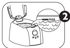
Then, using a jug, fill the stainless steel tank with normal tap water. The liquid must cover the object that is to be cleaned, but must not exceed the mark indicating the maximum filling height.
