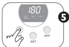
Press ON switch and start the cleaning process. The blue indicator lamp in the housing lights up while the time shown in the display counts down to 0.
